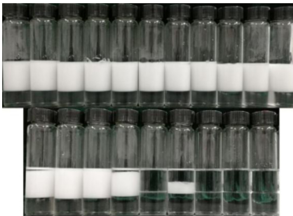
Fig. 6. OA-12-only emulsions with a concentration range from 0.014 to 4.378 mol·L -1 . The concentration decreases from left to right and up to bottom.
